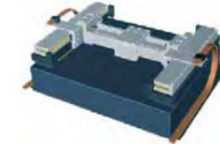
Air Bearing is applied for non-touching moving structure
